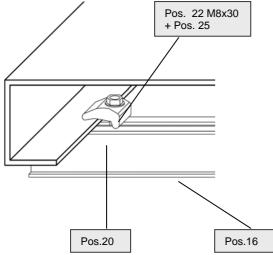
Both the clamp MTH and the bolts will have to be assembled with a sliding nut as shown beside. The sliding nuts have to be mounted in that way the side with the sharp, not rounded angles is pressed against the Aluminium profile.
